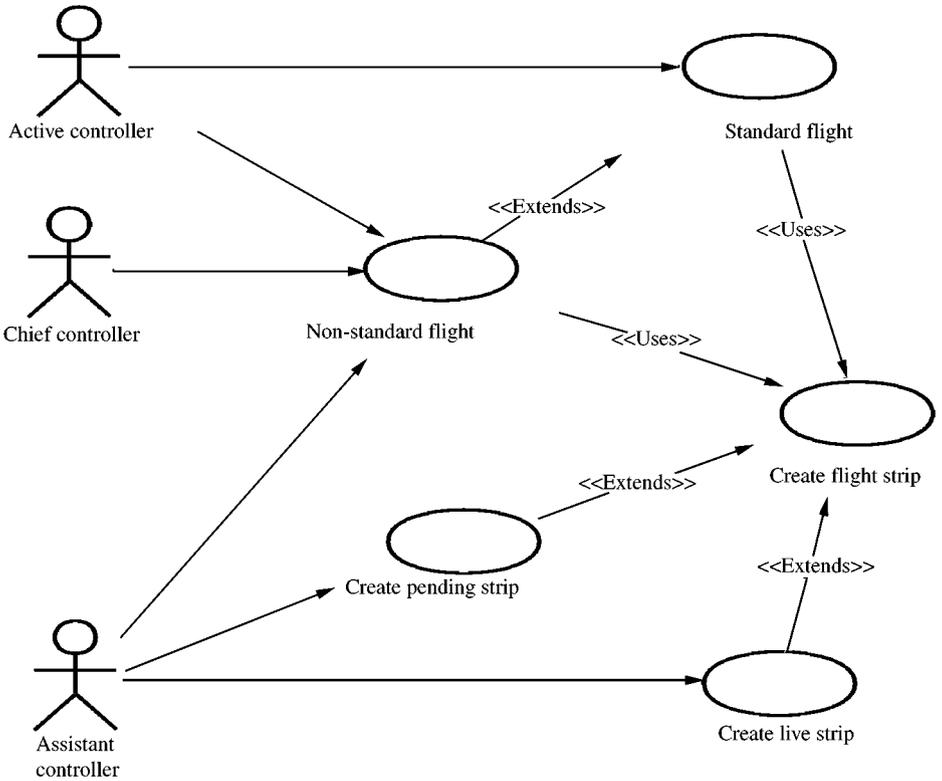
FIGURE 5. Initial use case model for ATC example.
