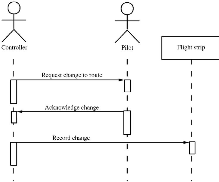
FIGURE 7. Sequence diagram for abstraction of flight coordination.
