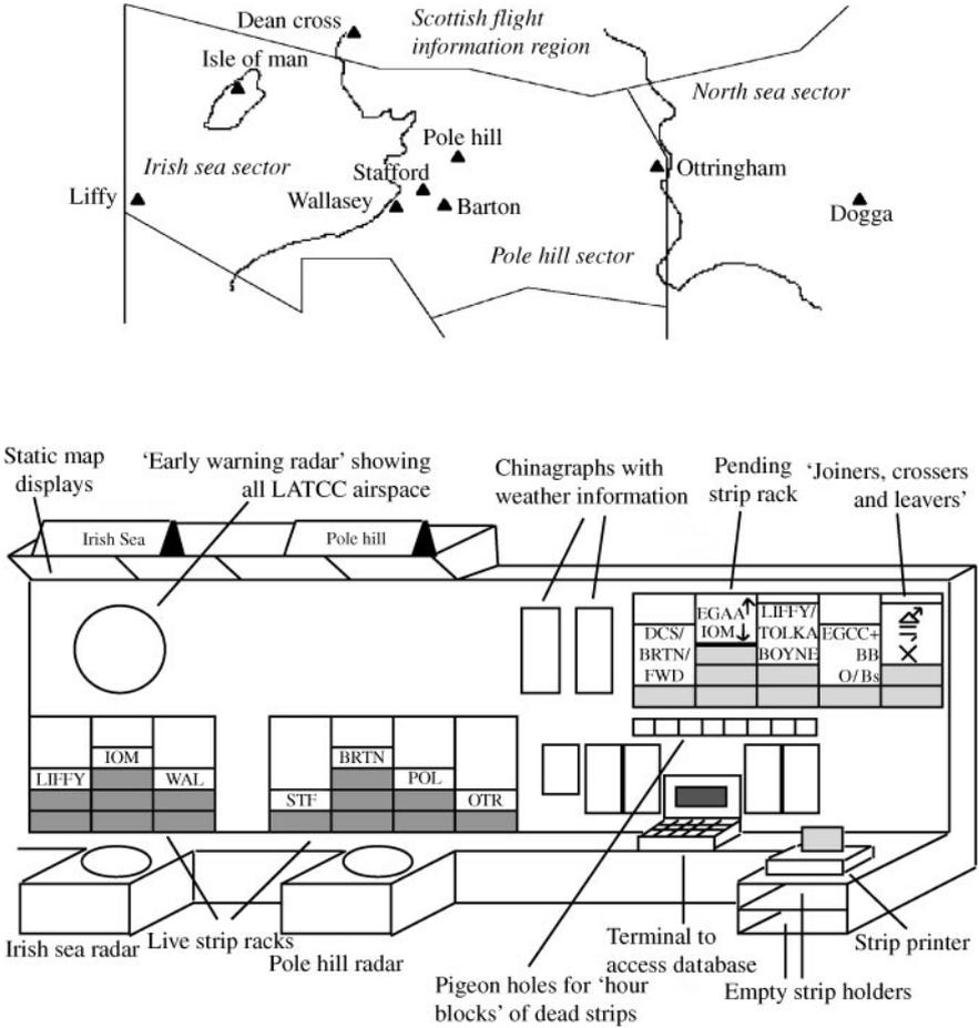
FIGURE 3. Simplified arrangement of Pole Hill Suite and Map of Pole Hill Sector<sup>2</sup> (from Hughes, Sharrock, Rodden, O'Brien, Rouncefield & Calvey, 1994b). The figure is simplified and not to scale. The map is included to show how the physical layout of suites and the order of the racks containing flight strips correspond to the geographical locations they represent. ■ Live flight strip; □ Pending flight strip
